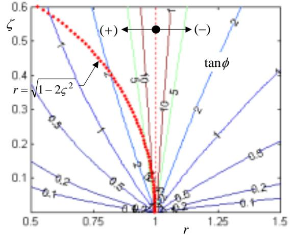
Fig. 1 Damping ratio  $\zeta$  vs.  $r$  and  $\tan\phi$ .
