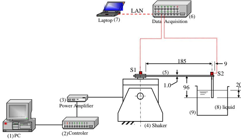
Figure 4. The experimental set-up (1: PC; 2: signal controller, Dactron; 3: Power Amplifier, B&K 2706; 4: Exciter, B&K 4809, 5: Cantilever; 6: Acquisition system, iMC  $\mu$ -Musys; 7: PC and Software, FAMOS, 8: Liquid, and 9: Glass cup).
