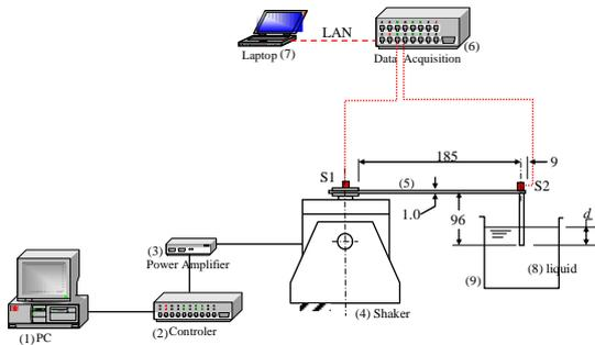
Fig. 7. The experimental set-up (1: PC; 2: signal controller, Dactron; 3: Power Amplifier, B&K 2706; 4: Exciter, B&K 4809, 5: Cantilever; 6: Acquisition system, iMC  $\mu$ -Musys; 7: PC and Software, FAMOS, 8: Liquid, and 9: Glass cup).
