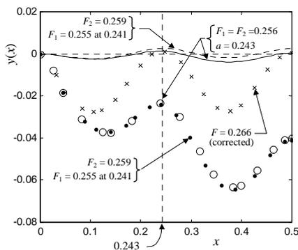
Fig. 11. Comparisons for the proposed model (Lines) and the FEM (Markers).
