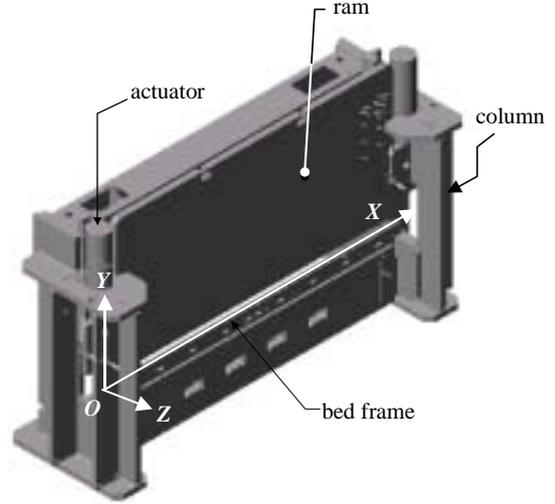
Fig. 1. A press brake and its coordinate system.
