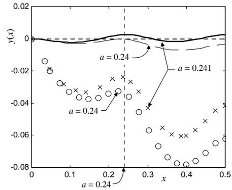
Fig. 9. Comparisons for the proposed model (Lines) & the FEM (Markers) for two different locations of  $a$  when  $F_1 = F_2 = 0.255$ .
