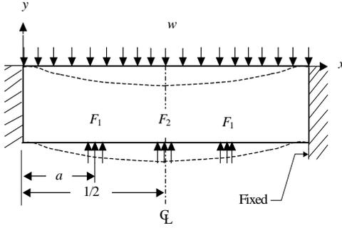
Fig. 2. Schematic diagram of the model for bed frames.
