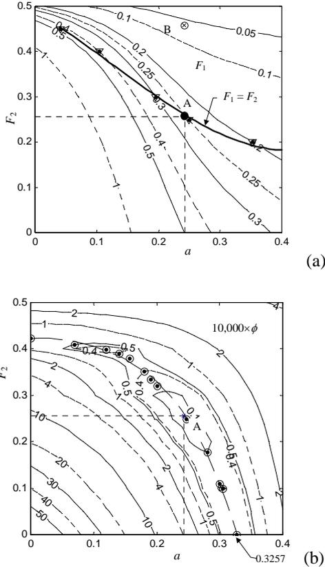
Fig. 7. Three-force compensation: (a) Optimal parameters; (b) Residuals.
