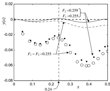
Fig. 10. Comparisons for the present model (Lines) & the FEM (Markers): (1)  $F_1 = F_2 = 0.255$  and (2)  $F_1 = 0.255$  &  $F_2 = 0.259$ .  $F_1$  located at  $a = 0.241$ .
