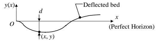
Fig. 3. Deflection of the bed along the  $x$ -axis.
