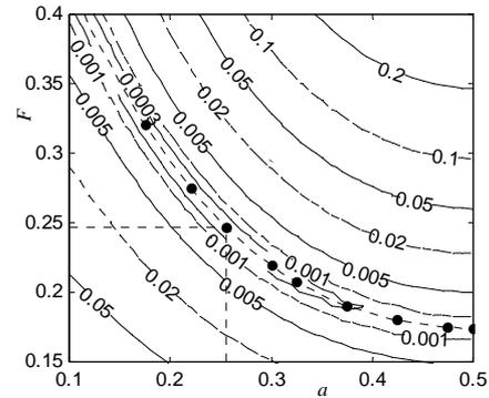
Fig. 6. The deflection residuals for three-equal-force compensation.
