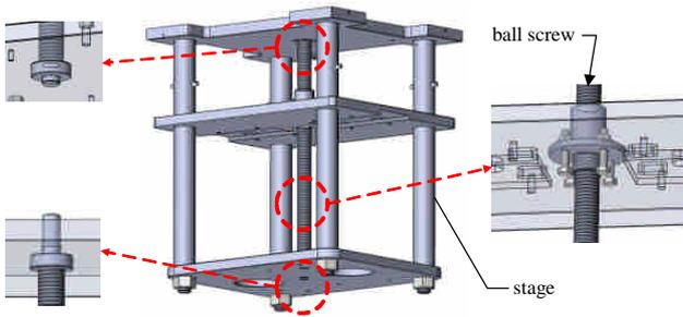
Fig. 11 The 3D model of the reciprocating unit.
