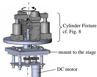
Fig. 10 The 3D model of the self-rotating unit.
