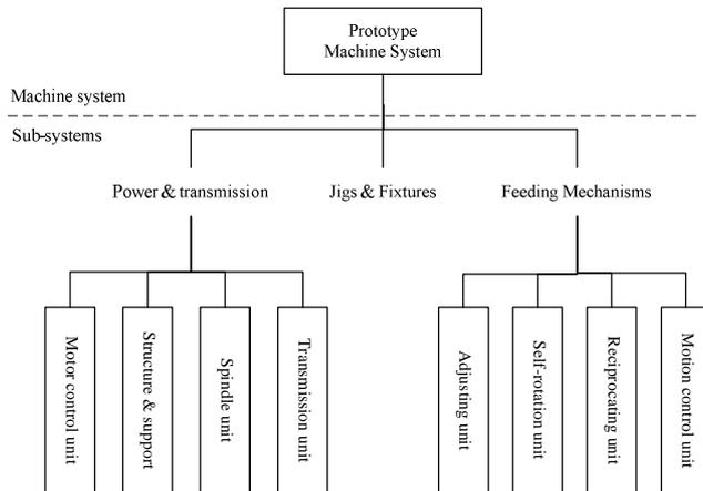
Fig. 4 The structure of sub- and sub-sub-systems of the polish machine.
