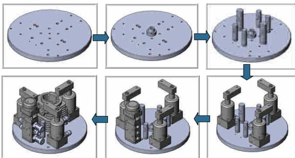
Fig. 8 The typical 3D assembling manual for the fixtures.
