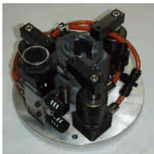
Fig. 13 The assembled pneumatic clamp.
