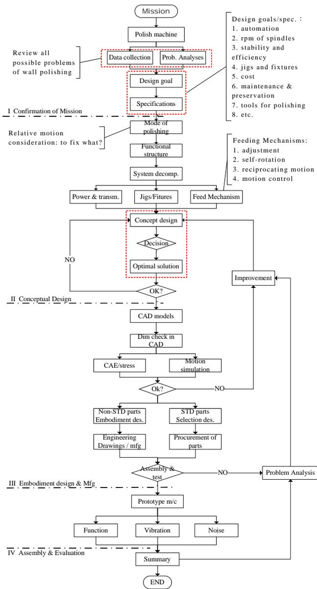
Fig. 2 The development flow of the prototype machine.
