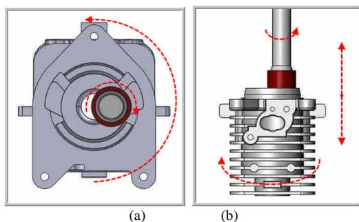
Fig. 5 The idea of 2 dof polishing mode: (a) relative rotational; and (b) linearly feeding .
