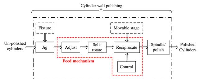
Fig. 3 The functional decomposition of the polish machine.
