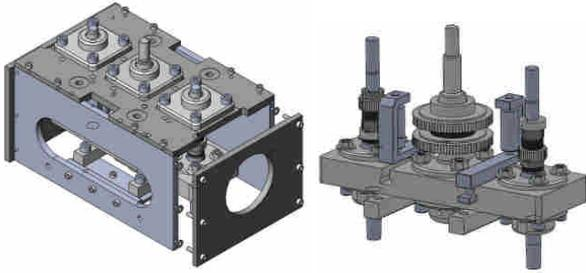
Fig. 7 Transmission unit: (a) Transmission box, and (b) The layout of spindle unit.
