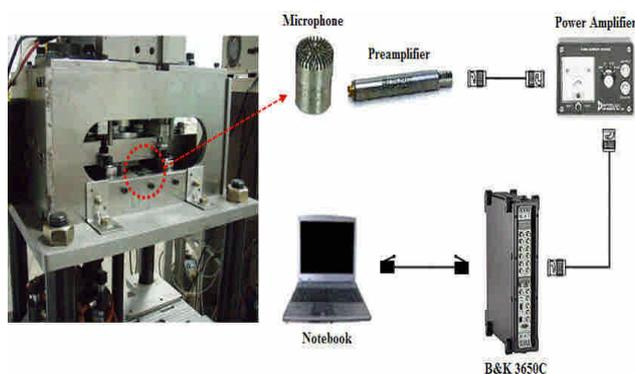
Fig. 17 The set-up of noise measurements.
