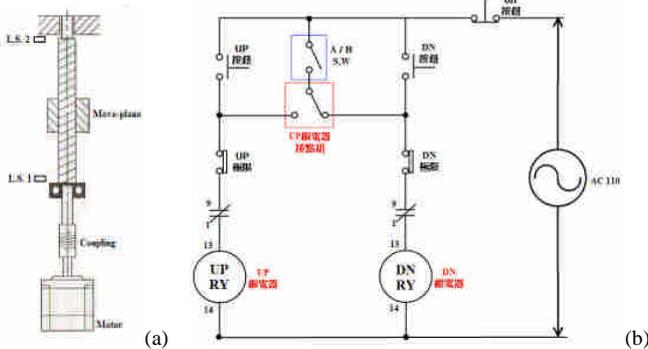
Fig. 12 The stage position control unit: (a) locations of LS and (b) their layout circuit.
