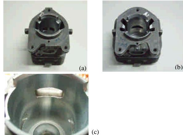
Fig. 1 Cylinders for lawn mowers: (a) 25 c.c., and (b) 30 c.c. before polishing; (c) polished inner wall.
