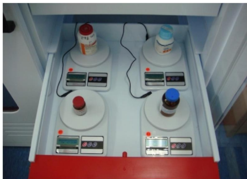
Fig. 11 Implementation of the multiple device system in the storage cabinet
