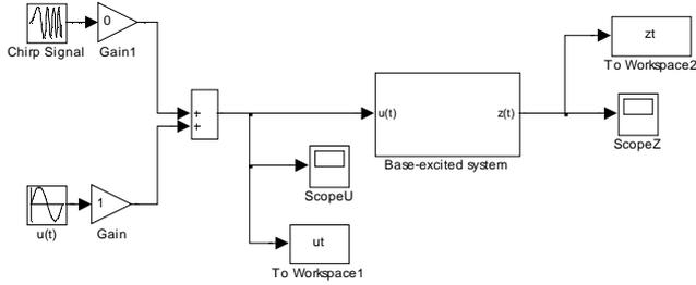
Fig. 2 The Simulink model for numerical verifications.
