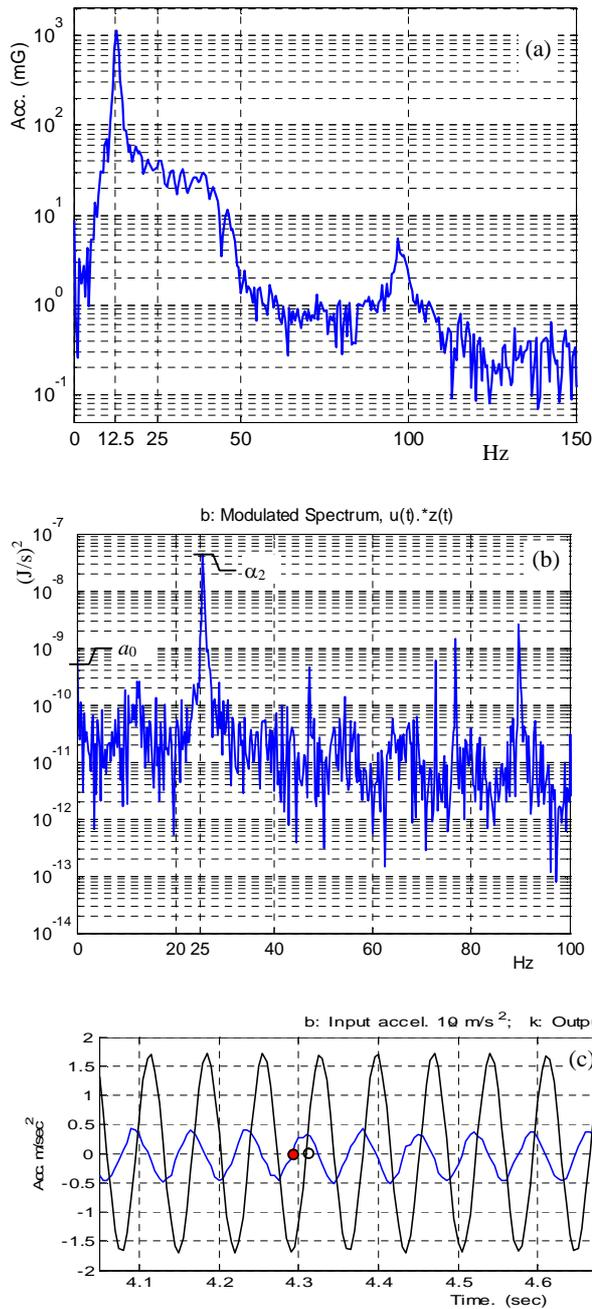
Fig. 4 Typical experimental results: (a) Frequency results from the chirp input; (b) Modulated signal where shows  $\alpha_2 \gg \alpha_0$ ; (c) Input excitation and output response in the time domain.
