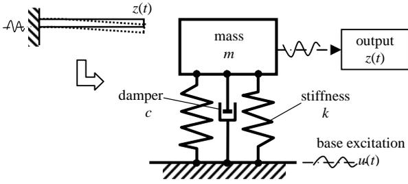
Fig. 1 A cantilever oscillator is modeled by a base-excited system.
