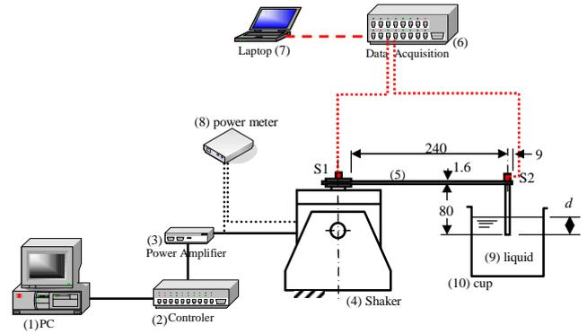
Fig. 3 The experimental set-up (1: PC; 2: signal controller, Dactron; 3: Power Amplifier, B&K 2706; 4: Exciter, B&K 4809, 5: Cantilever; 6: Acquisition system, iMC  $\mu$ -Musys; 7: PC and Software, FAMOS; 8: Power meter; 9 & 10: damper).
