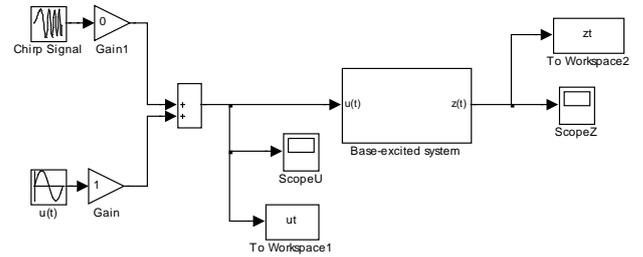
Fig. 3 The Simulink model for numerical verifications.
