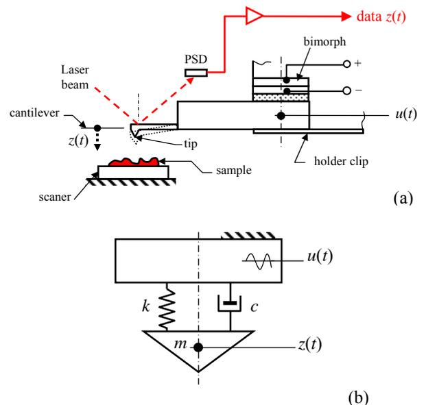
Fig. 1. (a) Schematic diagram of the optical lever detection system for an AFM; and (b) its dynamic model of the first mode.
