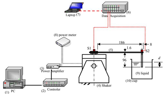
Fig. 4. The experimental set-up (1: PC; 2: signal controller, Dactron; 3: Power Amplifier, B&K 2706; 4: Exciter, B&K 4809; 5: Cantilever; 6: Acquisition system, iMC  $\mu$ -Musys; 7: PC and Software, FAMOS; 8: Power meter; 9 & 10: damper and liquid).
