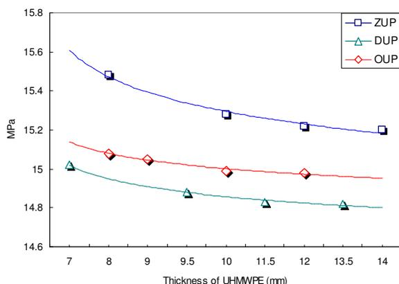
Figure 4. The max. von Mises stress on the PE tibial components of three different UKPs under various thicknesses.
