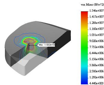
Figure 3. The max. von Mises stress is located at the center of contact area and occurs approximately 2 mm beneath the articulating surface.
