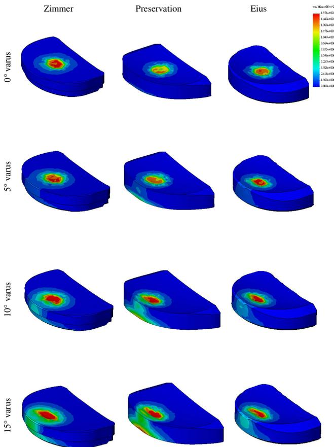
Figure 2. The contact patterns of the tibial PE components under various varus conditions for 5° posterior tibial slope.
