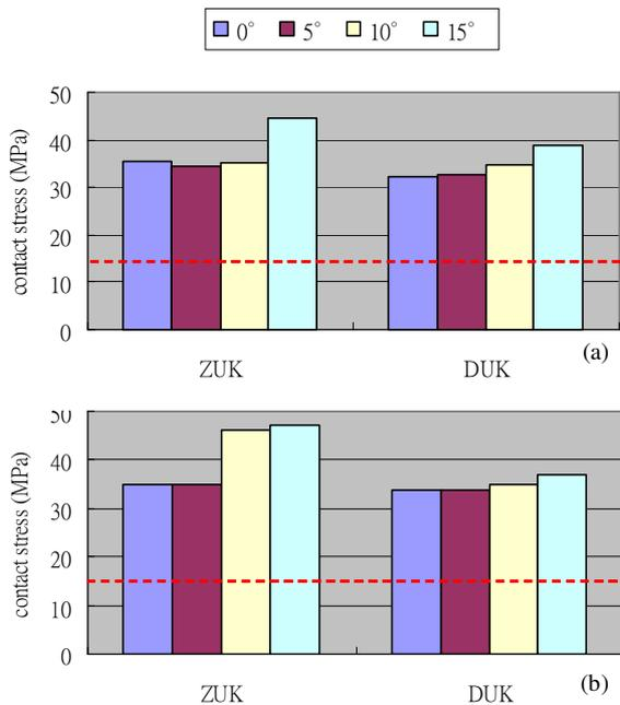
Figure 3. The max. contact stress on the PE tibial components of the two designs under the different varus tilt conditions for : (a) 5° and (b) 10° posterior tibial slopes.
