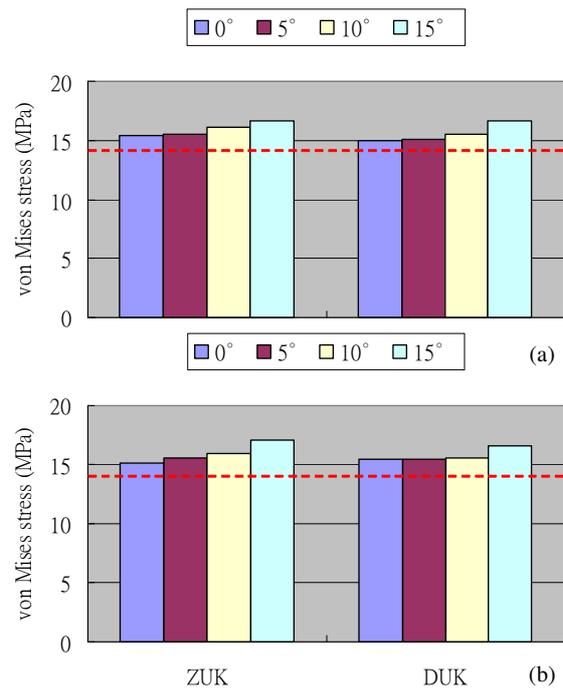
Figure 2. The max. von Mises stress in the PE tibial components of the two designs under the different varus tilt conditions for: (a) 5° and (b) 10° posterior tibial slopes.
