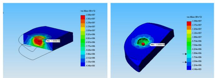
Figure 4. The max. von Mises stresses are located at the center of contact and occur approximately 2 mm beneath the articulating surface.
